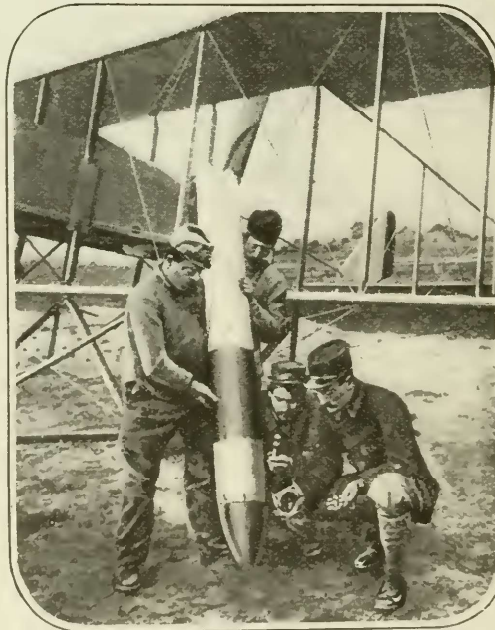
Modern "fletched" airplane bomb. Note streamline form, size, and weight, as shown
