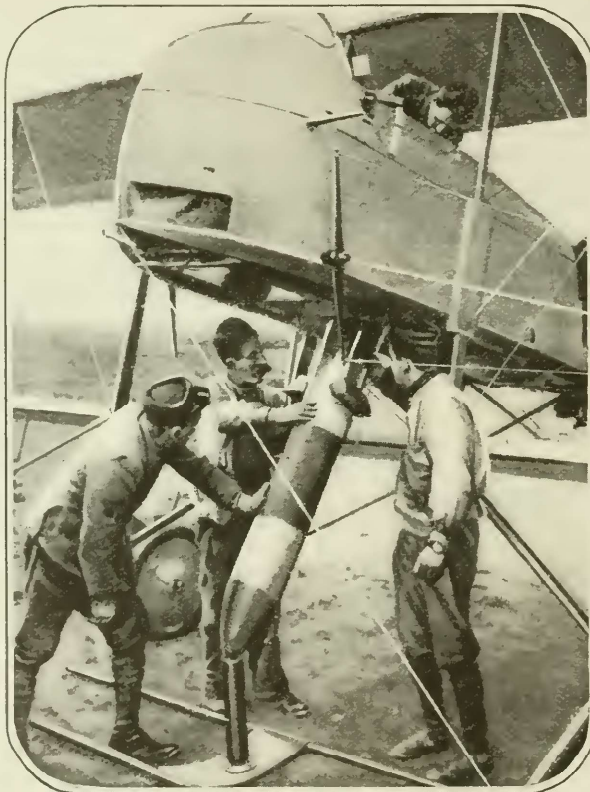
Slipping a bomb into an airplane. The tail is being inserted smoothly into the discharge tube
