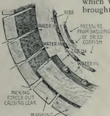
Showing how the pressure exerted by the swelling codfish forced the packing out of the planking, causing leaks
