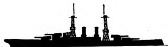
The length of these drawings indicates the difference in tonnage between ships of the Tosa class and the latest United States ships. The normal displacement of the Japanese ships is 41,800 tons compared with the 32,600 tons of the Maryland , one of the latest electrically driven United States fighting-ships
