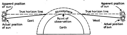
Because its rays are bent by the atmosphere, the sun appears to rise or to set when it is really below the horizon. A study of this diagram will make this clear to the reader
