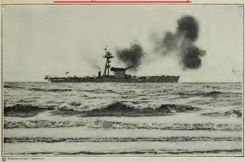
The first photograph ever made of one of the new British monitors in action. These craft are equipped with one fourteen or fifteen inch gun, and are very effective for coast bombardment. Six first-class monitors may be built at the cost of one super-dreadnaught, and are useful for coast attack as in the Dardanelles
