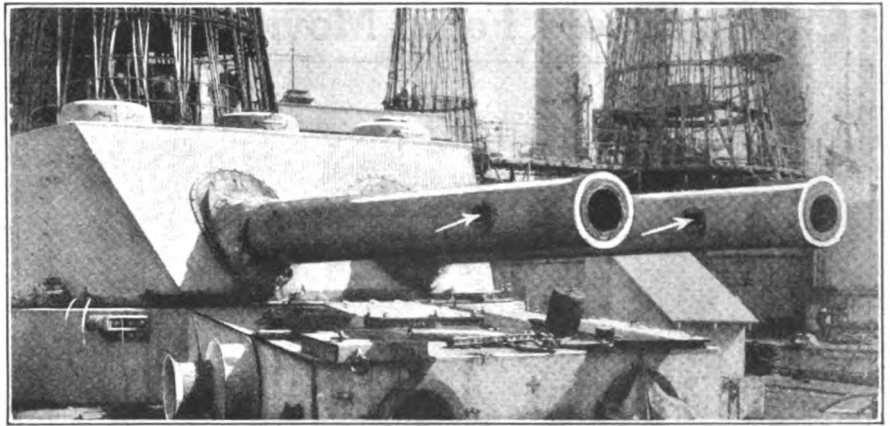
Arrows point to holes burned through 13-inch guns in the main battery of the battleship "Wisconsin" to prevent possibility of their use as deadly weapons
