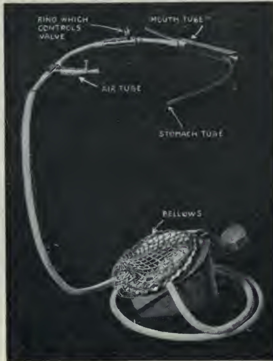
The apparatus consists of a throat tube, a stomach tube and a bellows, connected with the oxygen tank
