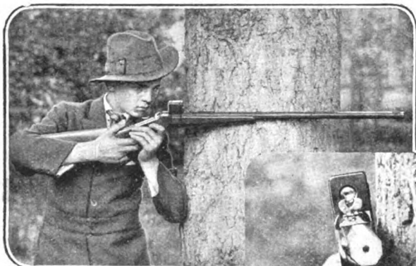
This sighting device enables the marksman to aim and fire behind cover. It is practically a camera finder applied to a rifle.
