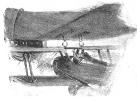
The 300-foot semi-rigid army airship "R-1" as she will appear when completed, with scout planes suspended from her rigid keel as explained below, and with navigation car forward and two power cars aft, side by side
