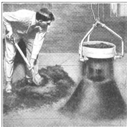
This sifter is shaken by an electric motor beneath the screen
