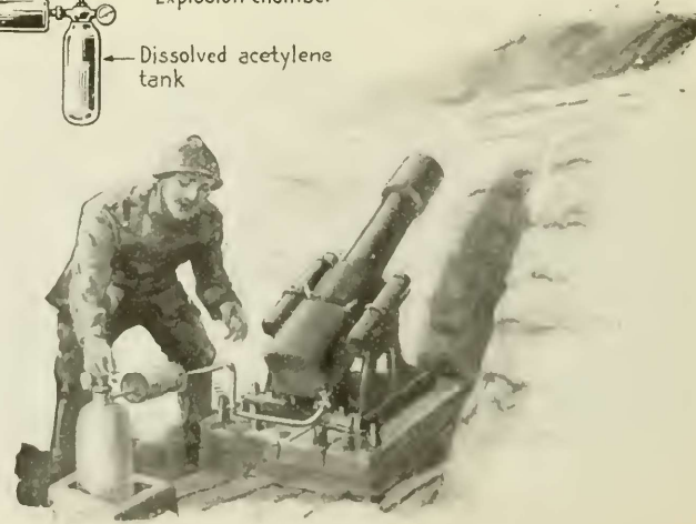
Diagram and illustration of a new acetylene trench mortar, fitted with silencer and recoil mechanism. Acetylene is too explosive for automobiles, but this is a virtue in guns
