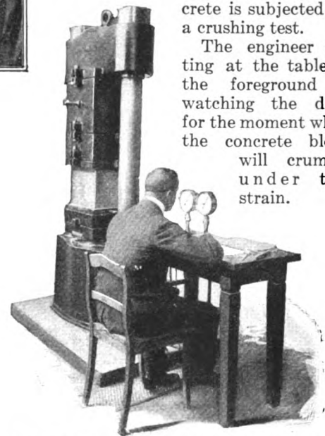
The resisting power of concrete is tested by a hydraulic press capable of exerting a pressure of four thousand tons to the square inch
