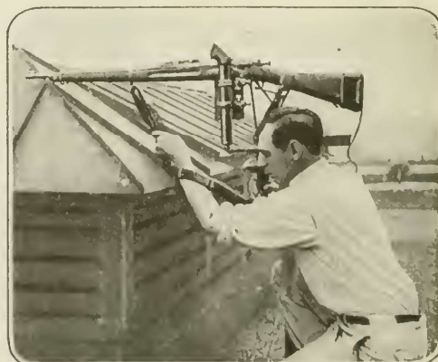
The trigger is pulled from the level of the shooter by means of an extension mechanism
