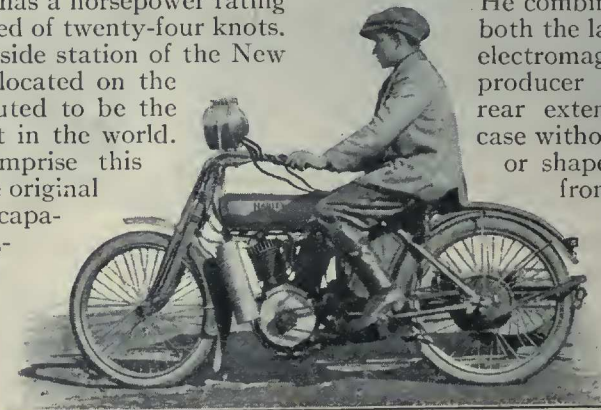
The motorcycle has many necessary accessories to carry so that a combination lamp and horn arrangement fastened to the handlebar saves valuable space
