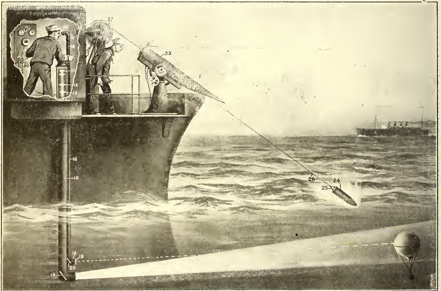
Latest Scheme for Locating and Destroying Submarines, Mines, etc., by Means of a Powerful Under-Water Searchlight and Periscope Device. Developed by Prof. Herschel C. Parker and Edward G. Hatch, M. E., of New York.
