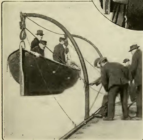
Pulling a lever in the center of the craft releases this life-boat upon reaching water
