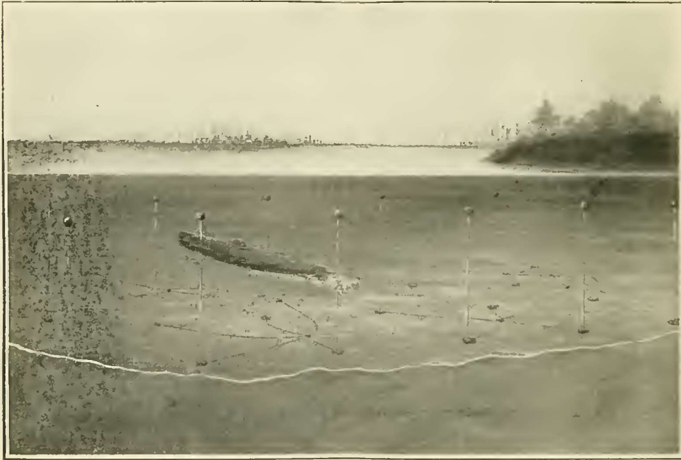
As a submarine progresses through a mine-field in the effort to reach shipping in a harbor, the hum of its electric motor is heard by microphones on the mines. The vibrations picked up by the microphones are electrically transmitted to shore and converted into visual signals by incandescent lamps corresponding in number and position with the microphoned mines
