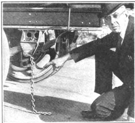
A dragging chain attached to the truck-frame carries off any static generated by filtering gasoline
