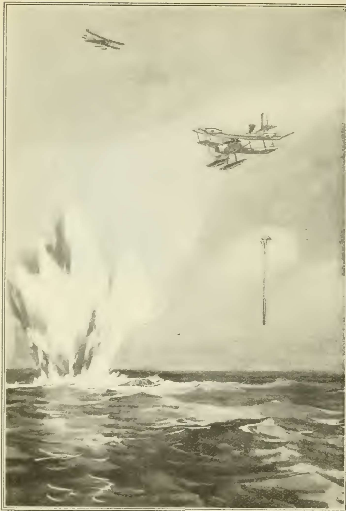
Hallock parachute depth-bomb. Flexible diaphragm, upon striking water, closes a pair of contacts. Circuit through the electric cable leading to bomb is thus closed; bomb explodes. Length of cable determines depth of explosion. If the diaphragm contactor fails to work, carbide contactors set off the bomb
