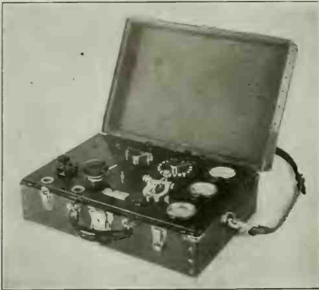
Extremely Light Weight, Portable Wireless Transmitting Set, Intended for Military or Other Purposes. It Operates on Batteries and Utilizes a Special Spark Coil and Quenched Gap. A Hot Wire Radiation Meter is Provided as well as Volt and Ammeter for the Primary Circuit.
