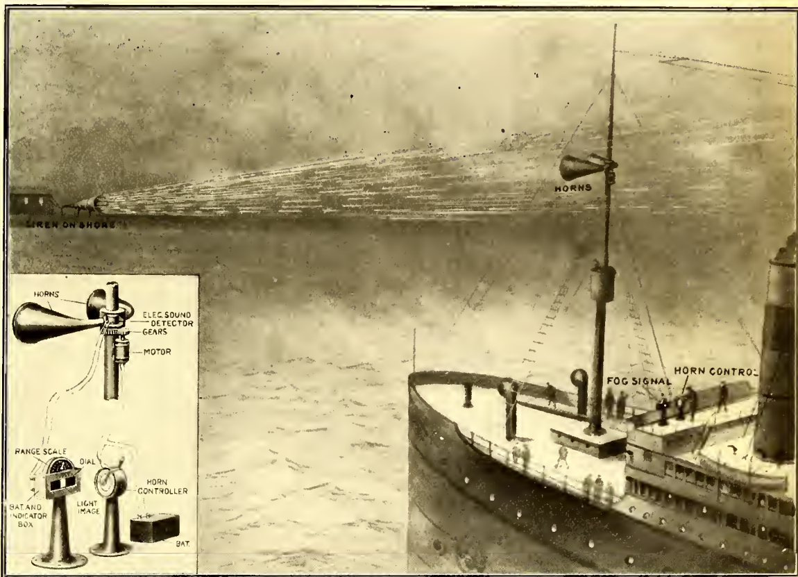
Remarkable Scientific Visual Fog Signal Receiver Devised by Dr. A. G. Webster, of Clark University. Insert Cut at Left Shows Details of Receiver Mechanism.
