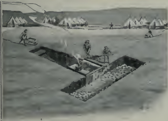
The refuse is burned on steel plates over the oven and the liquid drains off through the rocks
