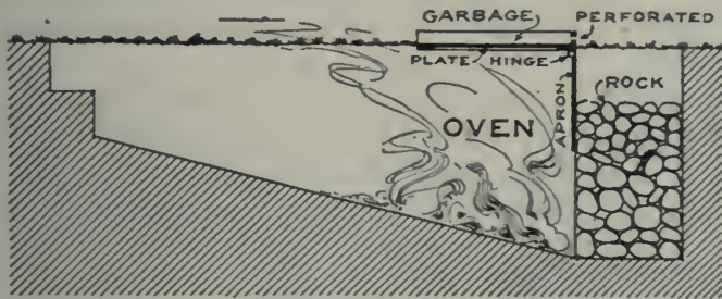
This incinerator can be built anywhere and disposed of quickly when no longer needed
