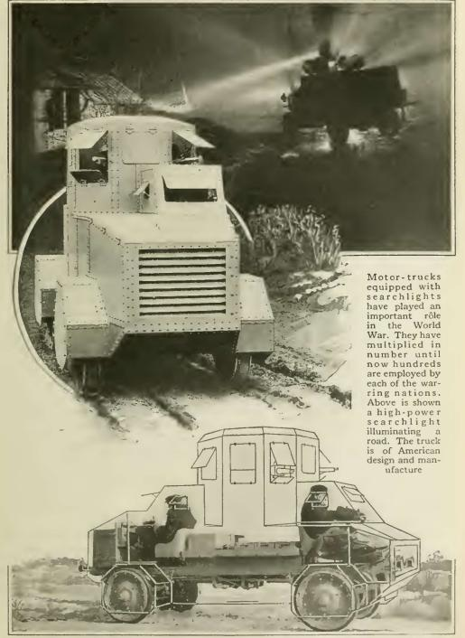
An American manufacturer has designed a truck operated from both ends. When beset by the enemy the crew need not turn around. The car fitted with an armor body is shown above at the left, while the stripped chassis may be seen below, the super-structure being drawn in faintly to show the positions of the drivers
