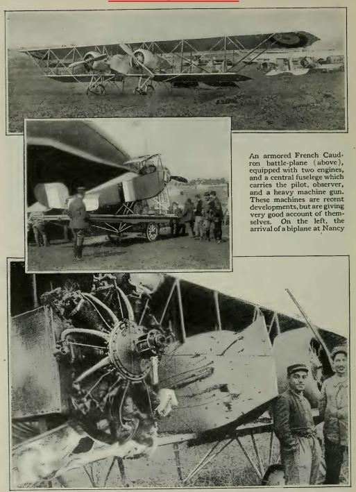
The result of a well-placed German shell, putting out of commission one of the Le Rhône rotary motors with which this machine is equipped. This is the same type of aeroplane as that shown in the illustration at the top of the page. Note the effects of the shrapnel upon the engine and the fuselege of the aeroplane
