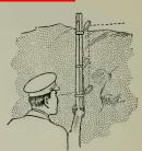
behind an intrenchment, can quickly attach this tiny instrument to the barrel of his rifle, to a pole, or to a trench-digging tool, and can readily observe, by means of the two circular mirrors, the movements of his antagonists in the distance without exposing himself to any tance without exposing himself.
