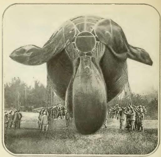
A captive sausage balloon is provided with auxiliary air-bags which serve to steady the balloon. In the latest form these give the structure the appearance of a huge elephant
