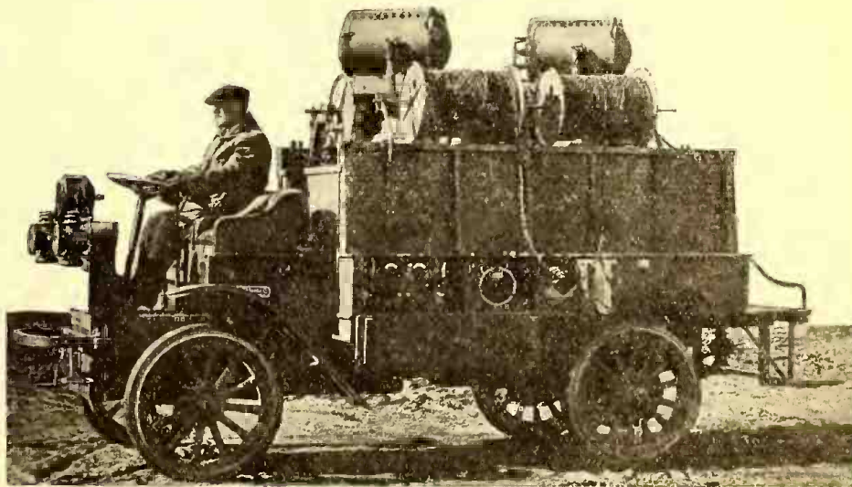
For Rapid Maneuvering of Troops at Night the U. S. Forces Will Have Available a Large Supply of These Auto-truck Searchlights.
