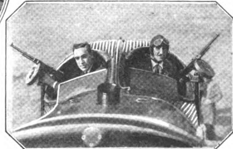
With three levers pilot and gunner control twenty-eight guns
