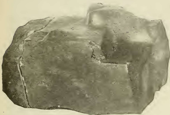
Papier-maché bomb made to resemble coal and filled with exceedingly high explosive
