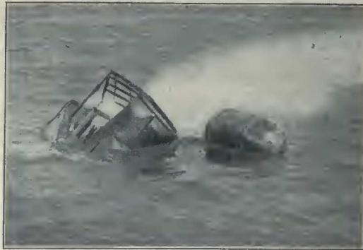
Ship in the act of sinking, showing two of the safes which have floated immediately to the surface
