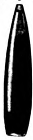
This 175-grain boattail bullet remained in the air 67 seconds; yet others of the same type, discharged at the same instant, stayed aloft 107 seconds, or 40 seconds longer
