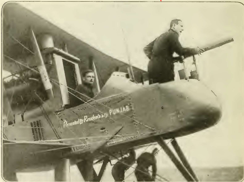
Maximum strength, minimum weight and least head-resistance are best attained by the aeroplane that has its propeller in front of a boat-body. But the propeller in front impedes observation. It also interferes with the operation of a machine-gun. Biplanes, such as this one, have been designed with the object of overcoming these military objections
