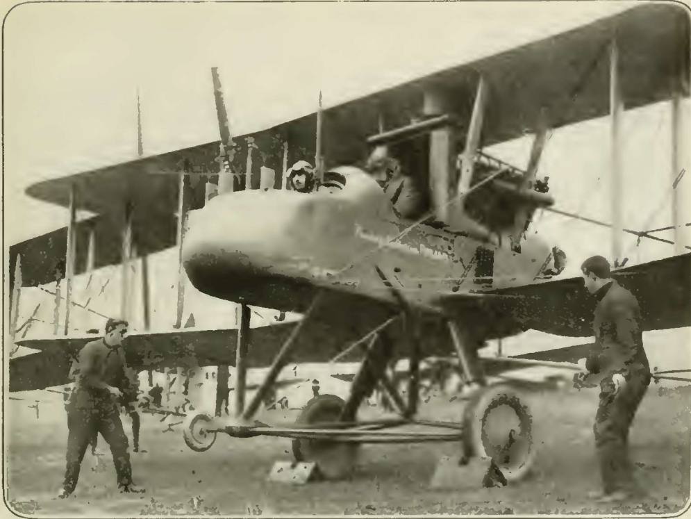
This British military aeroplane is of the latest type. And yet how similar it is to the crude, early machines of 1908. There are only two striking outward signs of improvement: the streamline boat-body enclosing everything and minimizing head-resistance, and the solid inflexible appearance of the wings, due to the invention of enamels which strengthen and shrink the cloth covering and make it as smooth on both sides as Japanese lacquer
