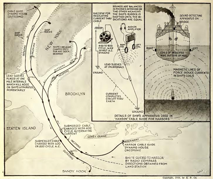
All During the World War There Were Hundreds of New Inventions Developed and Applied. One of These Was the "Hanson" Electrified A.C. Cable, Buried in the Mined Regions Where Our Ships Had to Travel. By a Suitable Listening Device Aboard the Ship the Navigator is Enabled Instantly to Ascertain Whether or Not He is Out of the Proper Course. A Great Stunt for Foggy Weather.
