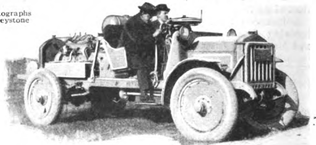
The gasoline motor that generates power to "fire" the gun, is mounted on the rear of a one-ton truck
