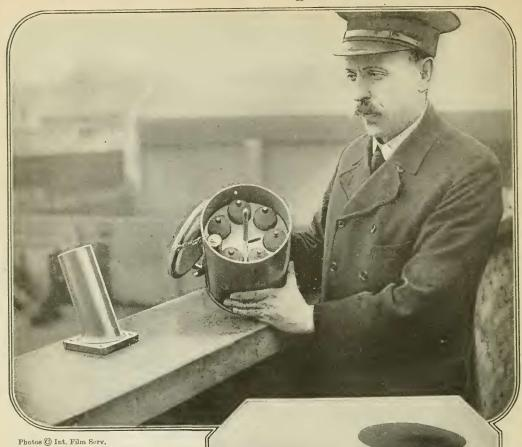
When air raiders approach London warning is now given by sound bombs which rise three hundred feet before exploding. Above is shown the mortar which is used for firing the rockets. They get results
