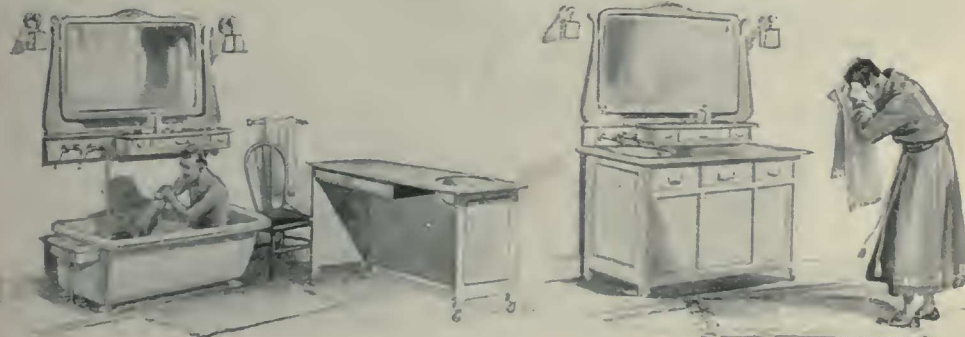
At left, the bathtub is shown in use, the concealing cover having been moved aside leaving the tub under the faucets, which are attached to a water-pipe through the stationary dresser-top. At right, the three parts of the device are united and an ordinary piece of furniture is the result
